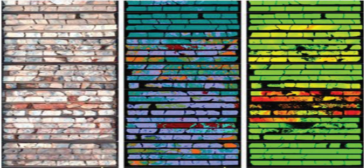
**Figure 34: Core Imaging Spectrometer**
